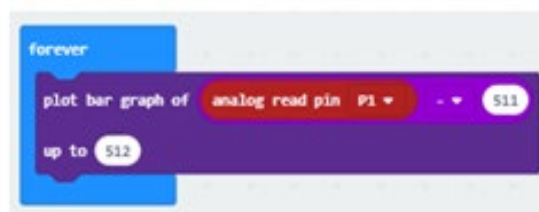
Image: sound level graph and visual coding used to collect the data with a micro:bit
